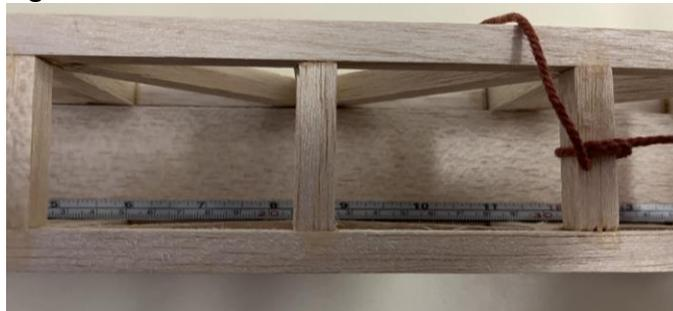
*Figure G1.1 Measuring midpoint of the road deck.*
